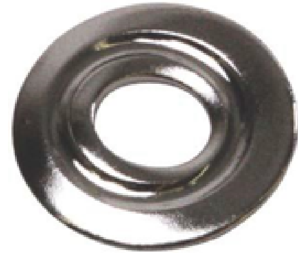
Over-tightened impression on a standard gasket after 1/2 turn. Note the distortion.
