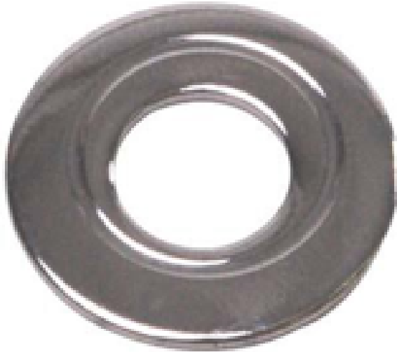
Impression on a standard gasket after proper tightening at 1/8 or 1/4 turn past finger-tight.
